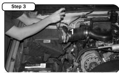
Diconnect and loosen the clamp on the MAF sensor (1). Remove the three 10mm bolts securing the air box. Disconnect the Temp sensor located on the side of the air box.
