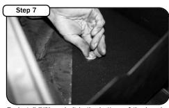
Re install 7/8"mm bolt in the bottom of the housing. Insert bolt thru the fenderwell and secure with sup-
