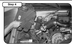
Lift up and remove the airbox assembly.
