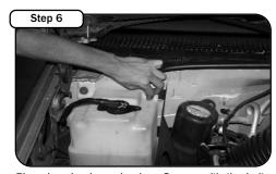
Place housing in engine bay. Secure with the bolts removed in step 5. Rear housing tab slips in behind
