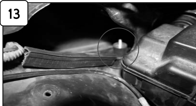
13 Install trim seal to fender cut-out. Install isolation mount to inner fender well.
