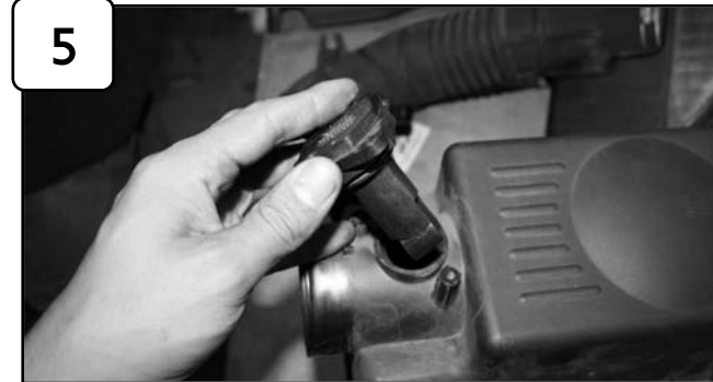
With phillips screwdriver loosen and remove MAF sensor.
