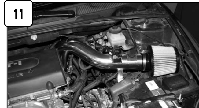
11 Install air filter and tighten using 5/16" nut driver. Tighten all clamps using 5/16" nut driver. Attach pre filter to filter if desired. Your short ram intake is now complete.
