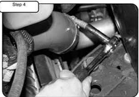
Loosen clamps on the intercooler elbow coupler using 7/16" deep socket with extension.
