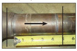
Step 7: Install the aFe direct fit catalytic converter replacement using the OE V- band clamp, but do not tighten. Slide the adapter pipe over aFe direct
