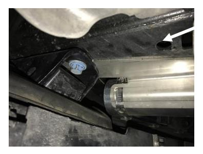
18. Place the reservoir in the bracket and tighten the hose clamps. Hose clamps should be placed through the openings in the bracket.
