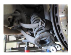
1. Install the factory upper spring seat, onto the new coil spring. Correct orientation would have the part number right side up. Raise the coil into the vehicle, positioning the upper seat into the hole in the chassis.
