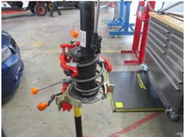
2. Install the strut assembly into the vehicle by lifting into place, and positioning the upper mount to the body. Having a helper on hand, reinstall the (3) upper bolts using a 13 mm socket. Torque to 25 lb-ft.
