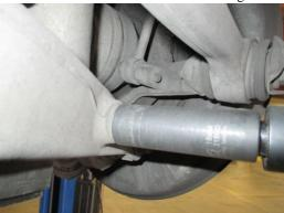
7. Using a 21 mm wrench and socket, remove the bolt holding the lower control arm at the upright. Slowly lower the control arm to release tension on the OEM springs, and remove spring from vehicle.
