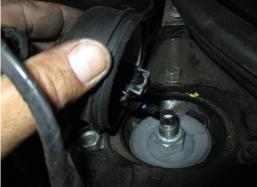
7. Using a strut compressor, remove the factory springs from the strut, by removing the top nut, using a 21mm 12 point socket.
