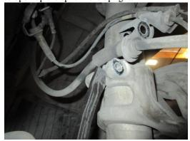
Using a 13 mm socket, remove the (3) bolts that hold the strut housing into the vehicle. Be careful to use a helper to hold the strut from the bottom of the car. If the vehicle is equipped with EDC shocks, you will need to disconnect the plug from the top of the strut.
