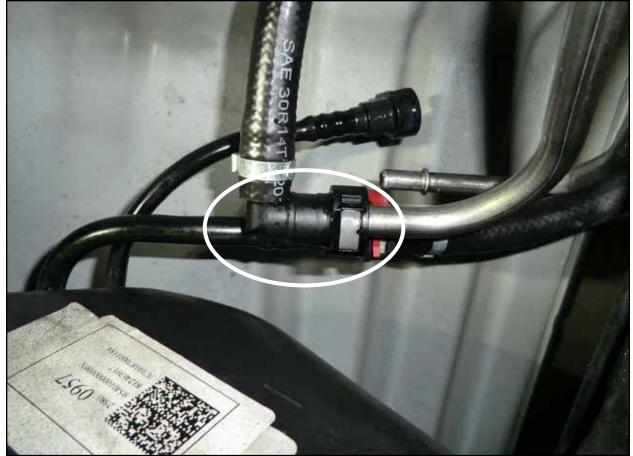
• Install the 90° female quick disconnect fitting on the supplied fuel outlet hose (black 90° -8 AN fitting shown below) onto the male side of the stock fuel feed line.
