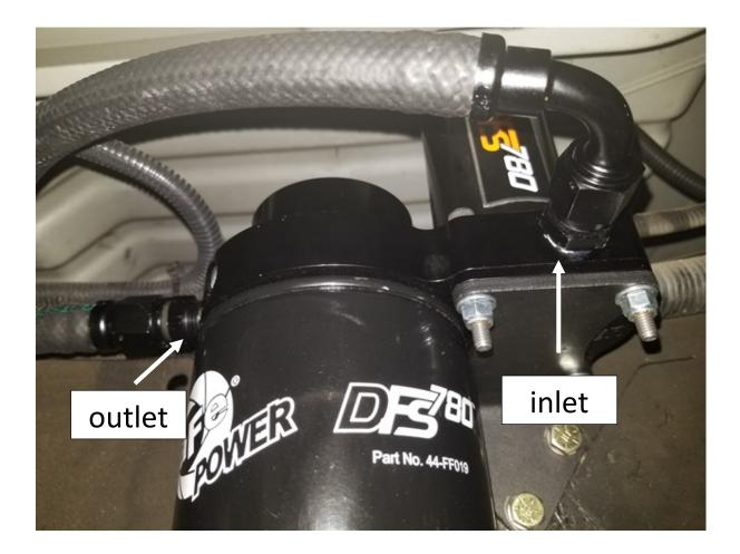
14. Attach the fittings to the inlet & outlet ports of the fuel manifold assembly. Make sure all connections are tight.
