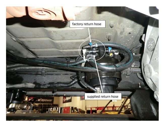
15. Disconnect the factory fuel return line. Attach the supplied fuel return hose between the male and female factory fuel fittings. Push all connections togethers.
