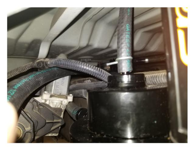
16. Carefully route the ¼" hose to the top of the air chamber on the fuel manifold assembly, making sure not to kink the hose or allow it near moving parts. Carefully mark and then cut the hose to the correct length. Using the supplied spring clamp, attach the hose to the nipple on the top of the air chamber on the fuel manifold assembly.
