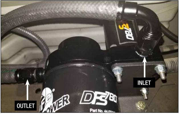
Step 13: Attach the fittings to the inlet & outlet ports of the fuel manifold assembly. Make sure all connections are tight.
