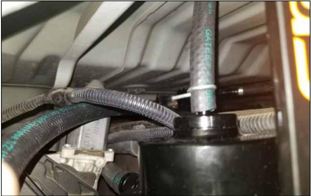
**Step 15:** Carefully route the ¼" hose to the fitting on the top of the fuel manifold assembly, making sure not to kink the hose or allow it near moving parts. Carefully mark and then cut the hose to the correct length. Using the supplied spring clamp, attach the hose to the nipple on the top of the air chamber on the fuel manifold assembly.
