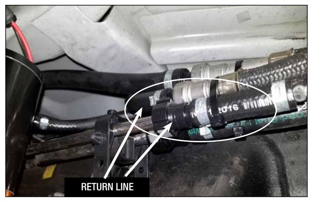
**Step 14:** Disconnect the factory fuel return line. Attach the supplied fuel return hose between the male and female factory fuel fittings. Push all connections together.
