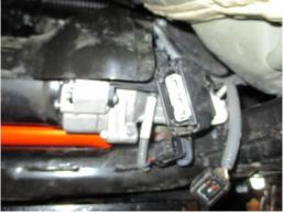
7. Secure the rear subframe, by re-attaching the left and right brackets. Shift subframe as required to keep everything aligned. Go back and torque the previously snugged subframe fasteners.
