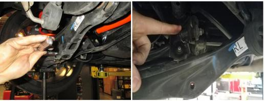
4. Remove the driver and passenger side sway bar mounts
