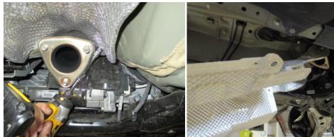
8. Once heat shield is removes from vehicle, disconnect the steering sensor connection. Disconnect steering rack connection on the side of the frame also.
