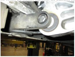
12. Re-secure the heat shield, and reinstall the exhaust
