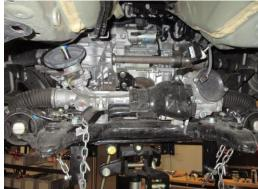
14. You can now access the steering rack bolts that hold the rack to the sub frame. Remove the 9 bolts that hold the rack to the sub frame.
