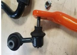
2. Grease inside surface and install new bushings onto the sway bar.
