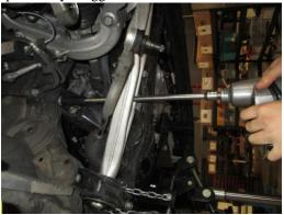
8. Reinstall the rear main subframe brace.
