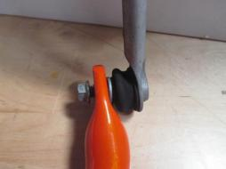
2. Reinstall the new sway bar by raising into the sub frame, in the pictured orientation.
