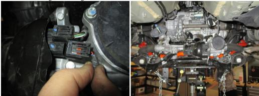
6. Raise the sub frame back up into its stock location and reinstall bolts and tighten down. Re connect all wiring to steering rack.
