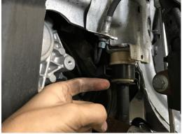
13. Slowly lower the subframe, be careful to ensure that you are not binding on anything and that all electrical connections and lines are free and not under tension. We were able to achieve this step by rotating the subframe back, and not completely dropping it from the vehicle. In this step be careful and make sure the steering spline does not get caught on anything.
