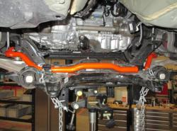
3. Reinstall the OEM brackets, carefully noting the correct orientation. Reattach the mounting hardware, and tighten bolts.
