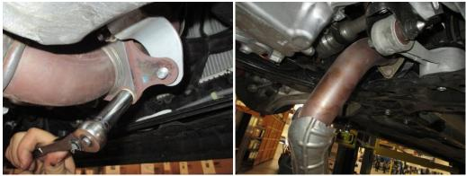
10. Loosen and remove the 19mm bolt that hold the engine mount. Remove sub frame braces using a 17mm socket.
