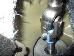
4. Use a 10mm socket to remove steering column bolt. **Before pulling the knuckle apart use a paint pen to mark the orientation of the two parts for proper column alignment later.**
