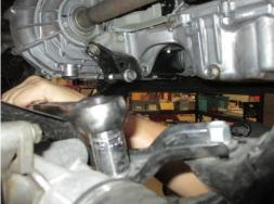
5. Reconnect steering rack wiring harness. This will complete the rack installment.
