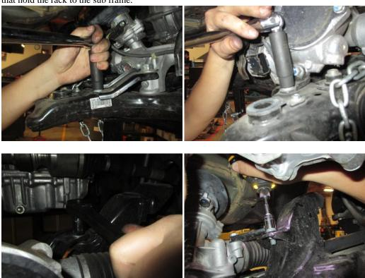
15. With the rack bolts removed you disconnect rack wiring harness. Now you can remove the whole rack from the sub frame.
