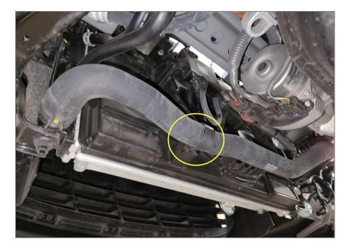
Unclip the radiator hose from the fan shroud.
