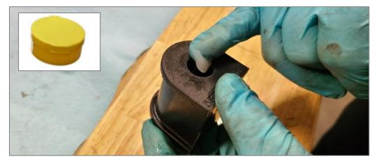
7R Open the bushing up and install onto the aFe Control sway bar.
