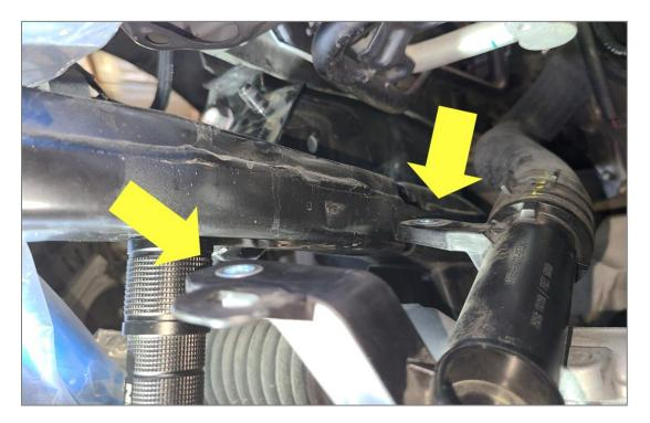
9F Unbolt the end links from the sway bar ends using a 14mm socket.
