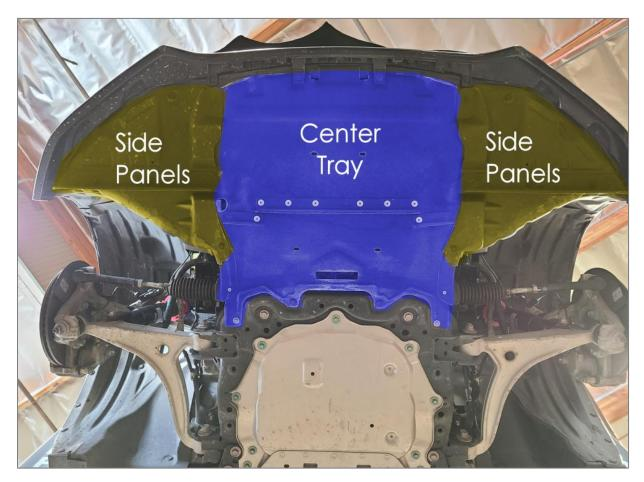
Unscrew and unclip all the fasteners below and inside the wheel well that secure the side panels and center tray using a slotted screwdriver and 8mm socket. Picture below shows the panels removed.
