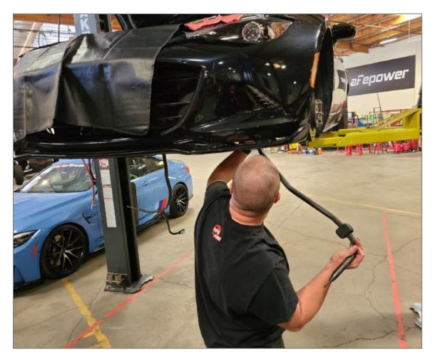
12F Familiarize yourself with the orientation of the sway bar. The bar ends will point towards to the rear of the car and the center hump should be up.
