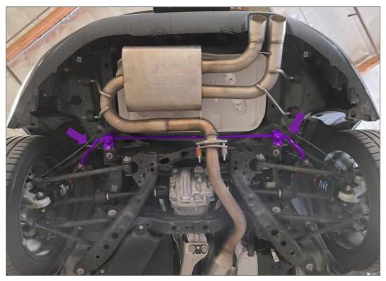
2R Unbolt the rear end links from the rear sway bar using a 14mm socket.
