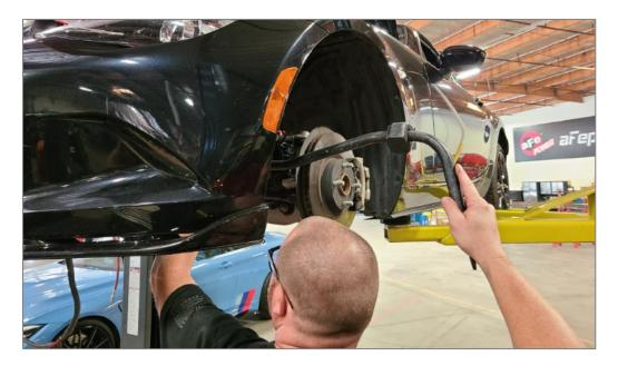
When you get to the 90° bend in the bar, rotate it downward to curl the bar out of the vehicle.
