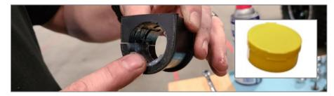
Open the bushing up and install on the sway bar.
