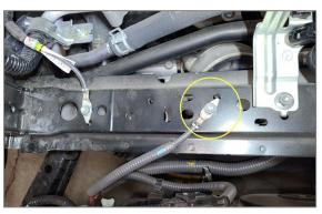
Some harness clips are easily disengaged by using a 90° pick and pushing the locking tabs in to release.
