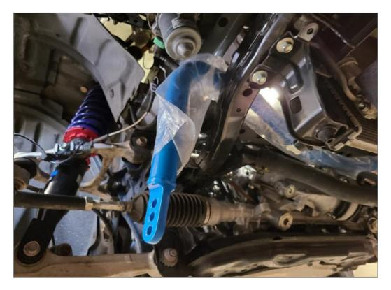
Rotate the bar so the ends can go over the steering tie rods and allow the bar to shift towards the back.
