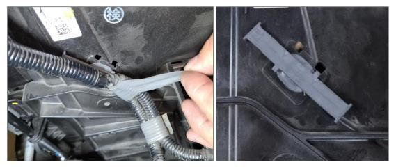
Unclip the harness hiding under the top radiator support. Pull the harness toward to rear of the vehicle.
