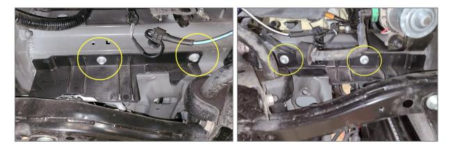
7F In order to get the front sway bar out, you will need to remove the fan shroud to gain more room. Start by disconnecting everything from the fan shroud.
