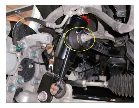
10F Unbolt the bushing brackets with a 14mm socket. Remove the bushing brackets so they are out of the way when removing the bar.
