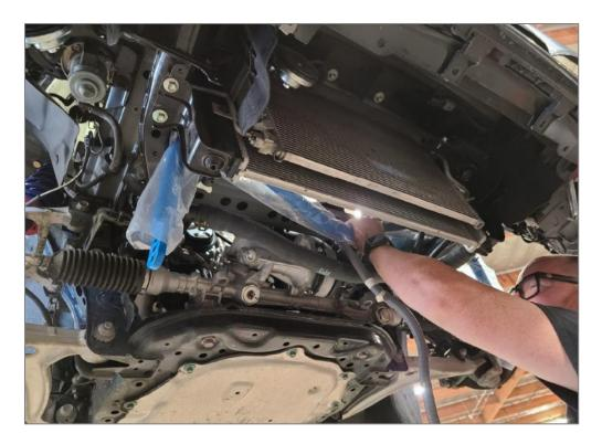
Bring the right side end up and over the subframe in between the subframe and unibody.
