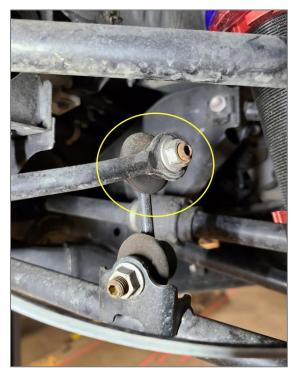
3R Unbolt the rear bushing brackets with a 12mm socket.
