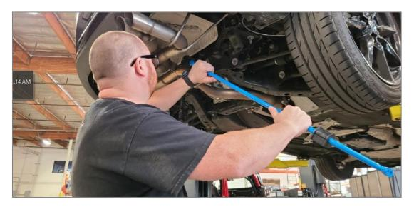
9R Install the afe Control billet bracket onto the bushings. Use the provided washers with the stock nuts and fully tighten.
