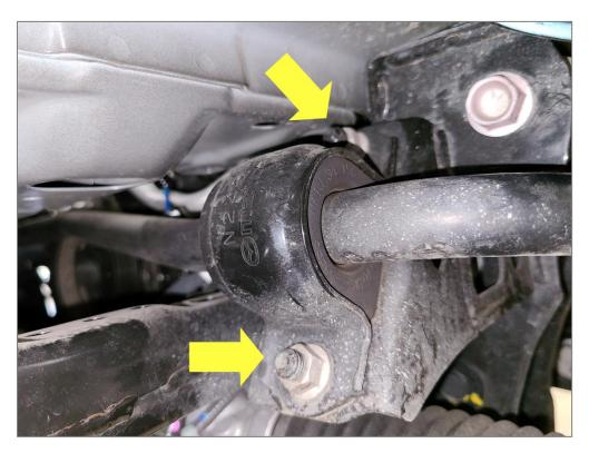
11F Fishing the bar out of the car will require a few steps. First, shift the bar forward so the arms clear the steering tie rods and can flop down.
