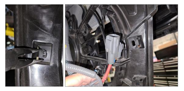
8F Follow the lower radiator hose and locate (2) bolted mounts to the subframe. Unfasten these (2) bolts.
