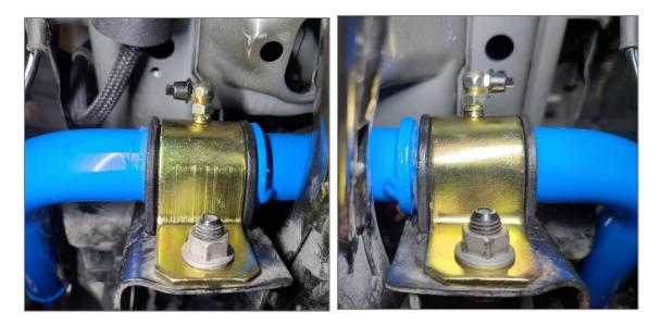
15F Install the end links onto one of three holes on your aFe Control sway bar. The hole closest to the end is the softest setting. (aFe suggest using the stiffest hole or the hole furthest from the end) Fully tighten this hardware.
