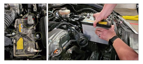
Unbolt and remove the battery tray with a 12mm socket. Undo the wire harness clip.
