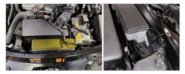
2F Next, remove the air intake box. Unclip the overflow tube from the box cover. Unplug the MAF sensor.
