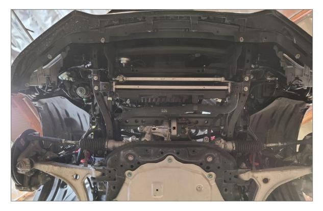
6F Next, remove the (2) plastic side guards attached to the frame rail near the sway bar bushings.
