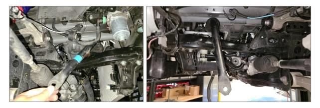
We will remove the bar from the left (driver) side so lift the passenger side end up through the gap between the unibody and the subframe.
