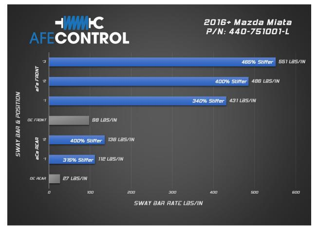
Stiffer roll resistance will demand more from the tires. When the tire's grip is overloaded, they will begin to slip. Manipulating when the front or rear tires slip can make the vehicle understeer, oversteer, or handle neutral. So, think of it as the higher the stiffness, the earlier the slip. If the front slips first, you will have understeer. If the rear slips first, you will have oversteer. If both front and rear slip near the same time, you will have neutral handling.
