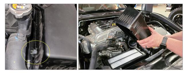
Unclip the MAF sensor harness from the cover. Remove air filter and unbolt air box housing and set aside.
