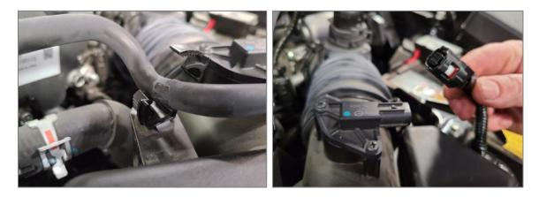
Loosen the clamp connecting the rubber hose to the air box.
