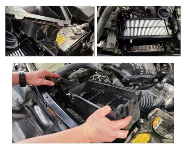
3F Remove the battery by disconnecting the negative and positive terminals and hold down bracket using a 10mm wrench.
