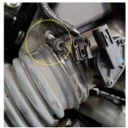
Unclip the air box cover and lift up.
