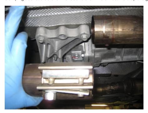
Remove the exhaust system that is fully disconnected now.
