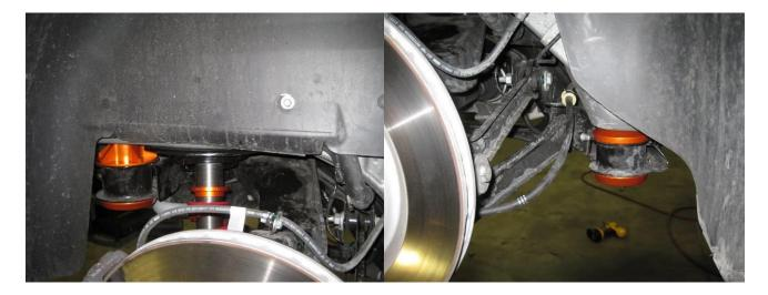
7) Re-install the brake calipers, e-brake lines, driveshaft, lower shock mount and electrical connector
