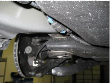
9) Disconnect the driveshaft flange on differential from the driveshaft. These are 18 mm in size.
