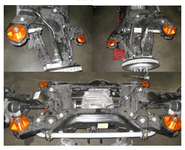
3) Lower the body back on the subframe being careful to align the pins on the body into the mounts.
