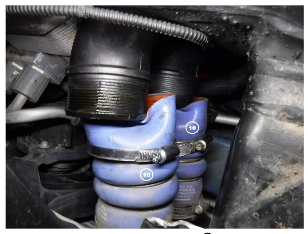
14. Loosen the clamps securing the hot side intercooler tubes 10 to the intercooler on the passenger side of the vehicle.
