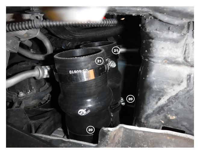
Note: Be sure to thoroughly clean all oil residue off of the connections before installing the supplied aFe couplings onto the vehicle
