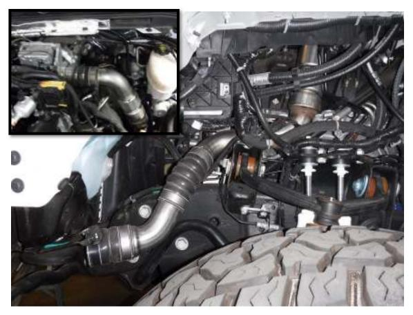
72. Reinstall the factory hot side intercooler tube into the vehicle from the bottom. 73. Ensure the tube is not touching anything then tighten all the clamps using an 11mm socket.
