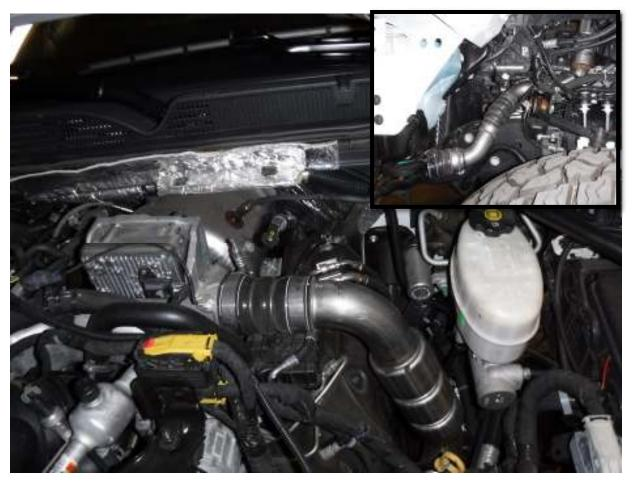
20. Loosen the clamps for the hot side intercooler tube at the turbo outlet and intercooler inlet on the driver side of the vehicle using a 11mm socket.
