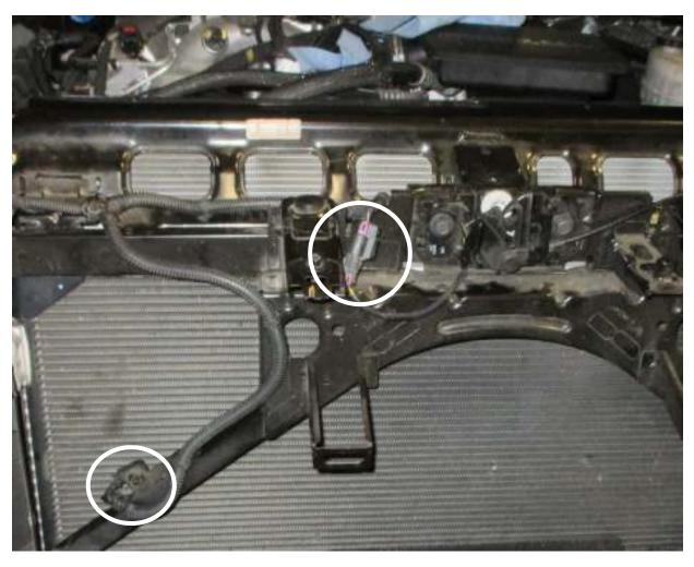
34. Disconnect the temperature sensor and hood latch from the wiring harness. 35. Unclip the wire harness from the core support and set aside.
