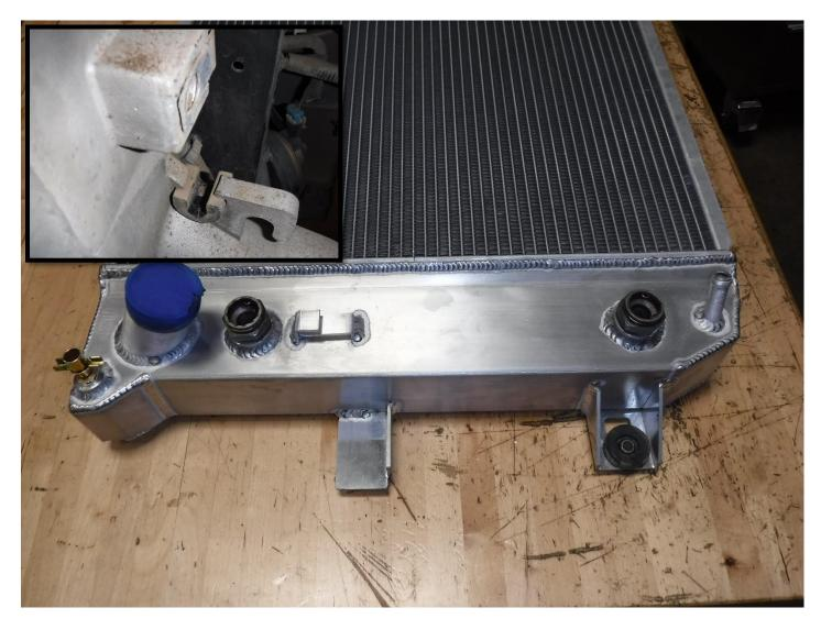
Note: Be sure to lubricate the O-rings with grease to prevent them from tearing during installation.
