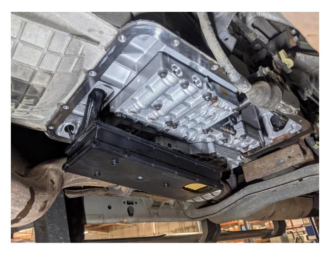
14. Install the supplied aFe transmission filter.
