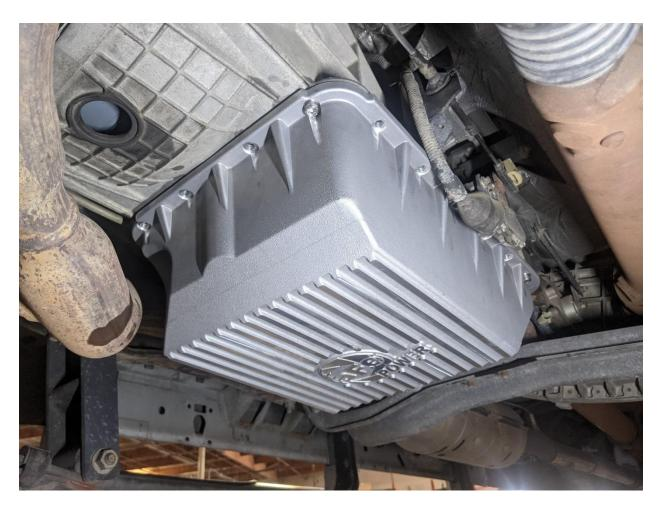
19. Hold the transmission pan up into position, aligning the screw holes. Install four (4) M8x1.25x20 socket head screws and M8 screws into each of the corners to hold the pan into position.
