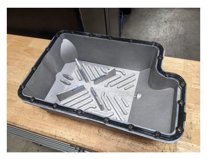
16. Hold the supplied aFe transmission pan up to the gasket surface to make sure you will be able to maneuver it into place.
