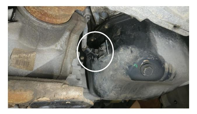
5. Disconnect the sensor connector and make sure that all wires are out of the way.
