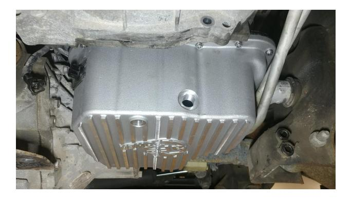
23. Hold the oil pan up into position, aligning the screw holes. Install four (4) M6x1.0x20 socket head screws and M6 washers into each of the corners to hold the pan into place.
