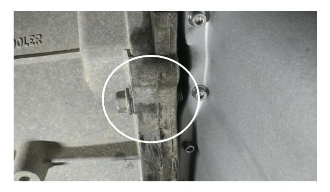
30. Re-install the transmission bolt removed in Step 11, using the supplied M10 washer.
