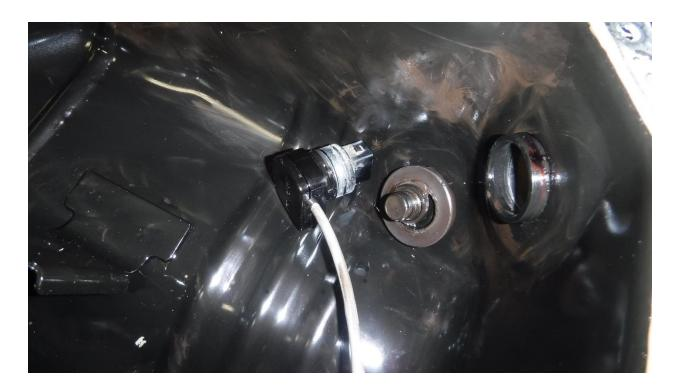
14. Once this holding clip is removed, push the connector towards the inside of the pan.
