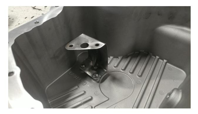
16. Prepare the supplied sensor bracket, oil pan, two (2) M6x1.0x12 button head screws, and two (2) M6 washers. Attach the sensor bracket to the oil pan using the M6x1.0x12 button head screws and M6 washers. Make sure the bracket is facing the correct direction as shown above.
