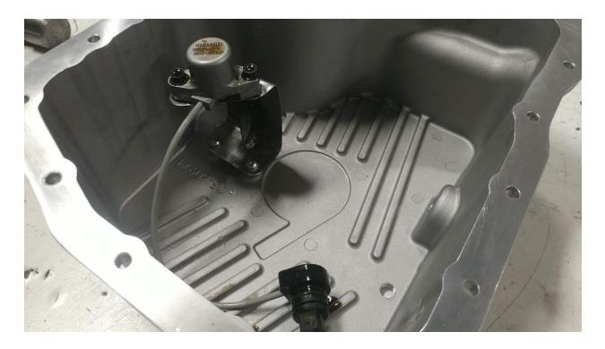
17. Install the sensor to the sensor bracket using the two (2) screws removed in Step 15 and the two (2) M6 nuts used in Step 9.
