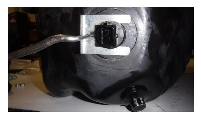
13. Pry the metal holding clip from the outside of the oil pan.
