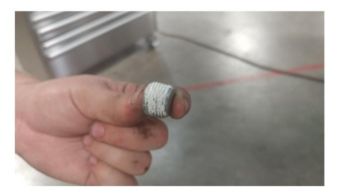
Note: If using an oil heater, apply Teflon pipe sealant to it instead of the  $1/2^{\prime\prime}$  NPT plug.
