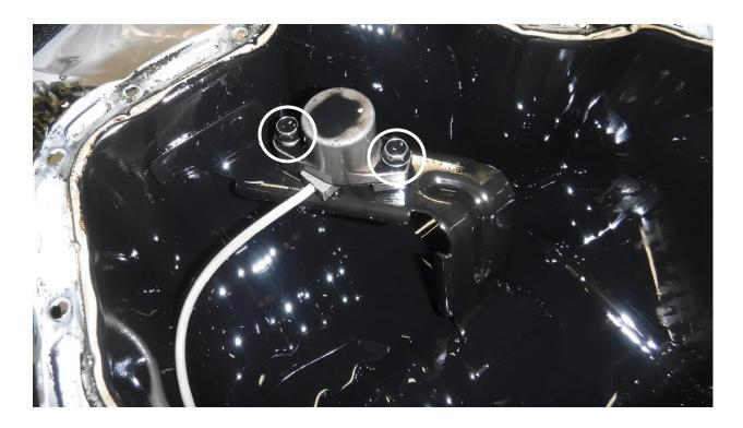
15. Remove the two (2) screws holding the sensor to the bracket inside the oil pan.
