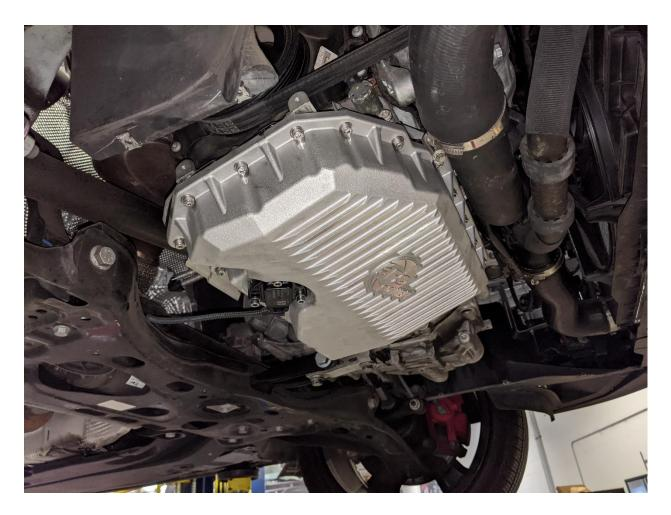
15. Hold the oil pan up into position, aligning the screw holes. Install one (1) M6x1.0x20 socket head screw and M6 washer into each of the four (4) corners to hold the pan into place.
