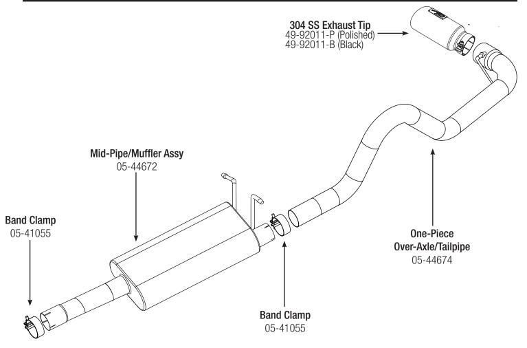
**Step 1: (Read Instructions prior to installation)** Remove your stock exhaust from the rear of your truck working your way forward. It may be necessary to cut the pipes if the slip joints are stuck. Do not cut the pipe after the cat. You will be using this slip connection. Take caution not to damage the factory isolation mounts, as they will be reused. It is recommended to not fully tighten the clamps until the entire system is installed.
