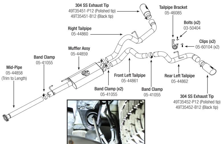
Step 1: (Read Instructions prior to installation) Remove your stock exhaust up to the catalytic converter from the rear of your truck working your way forward. Take caution not to damage the factory hardware and isolation mounts as they will be reused.
