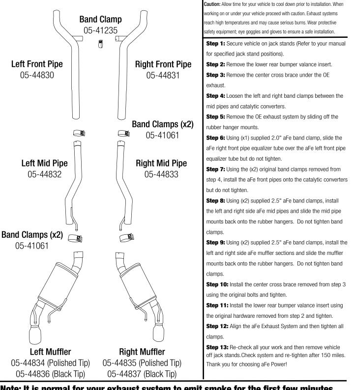
Note: It is normal for your exhaust system to emit smoke for the first few minutes upon initial start-up due to grease used in the mandrel bending process.
