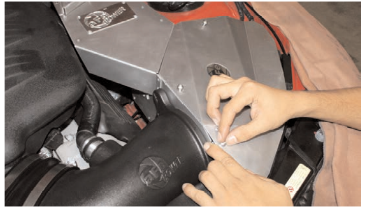
29- Secure cover with supplied M6 button head screws and tighten with 2.5mm allen wrench.
