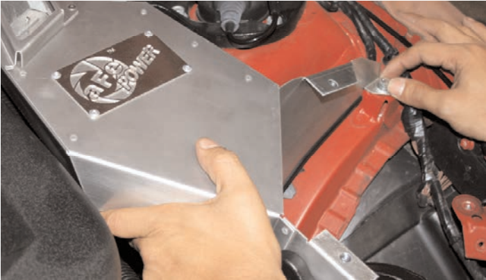
18- Install the supplied hex screw, wavy washer and flat washer into the upper mounting tab. Do not fully tighten
