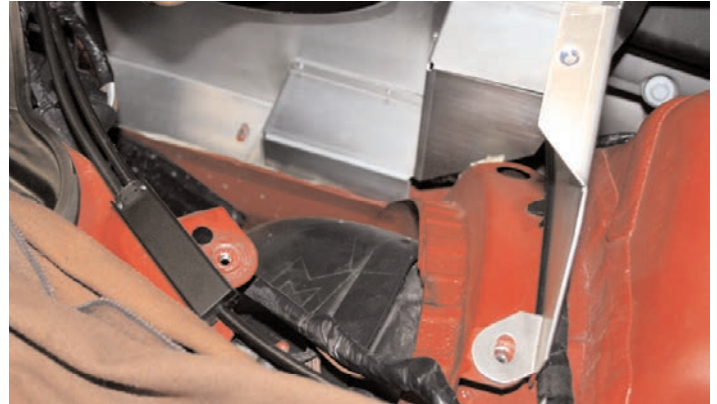
14- Carefully position housing into the vehicle and line up the mounting points.
