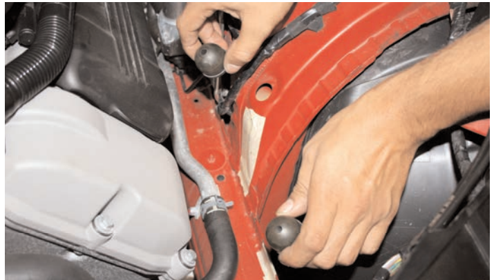
7- Remove the stock rubber mounts that are located under the stock intake box and put them aside.
