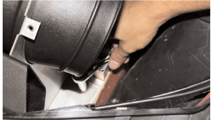
22- Tighten lower housing support nut with 10mm socket or wrench.
