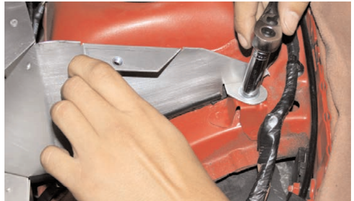
23- Once aligned, tighten down the upper mounting bolt with 10mm socket or wrench
