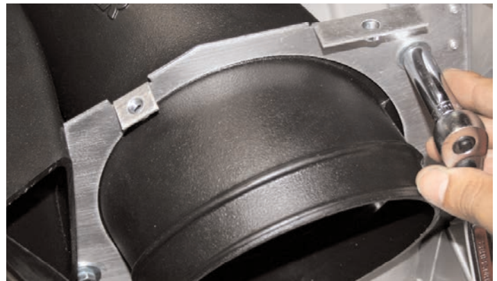
24- Tighten down the bolts installed in steps #10 & #11 using a 10mm socket or wrench.
