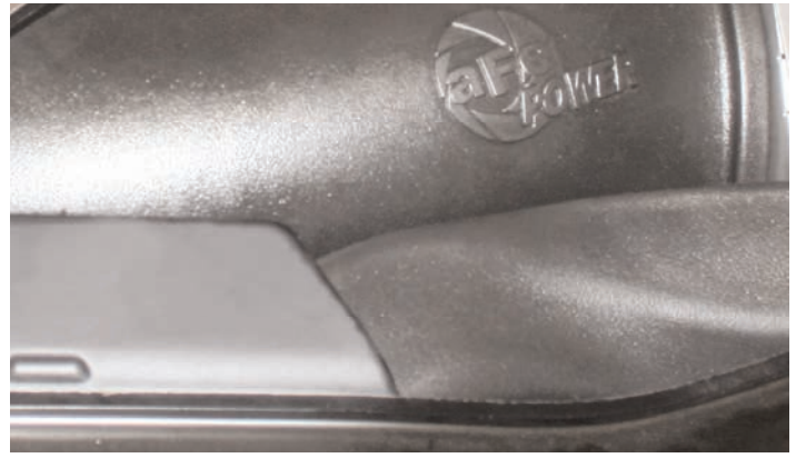
21- Once in position, push the cold air duct into the factory cold air inlet. It should fit snug to form a seal.
