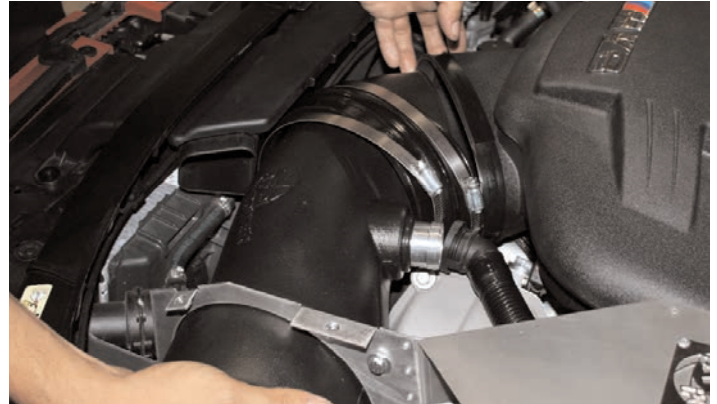
15- Line up intake tube with the intake plenum.
