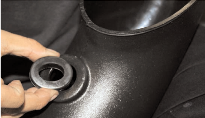
10- Install supplied grommet into aFe's intake tube.
