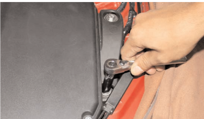
4- Remove the two airbox mounting bolts shown with 10mm socket or wrench.
