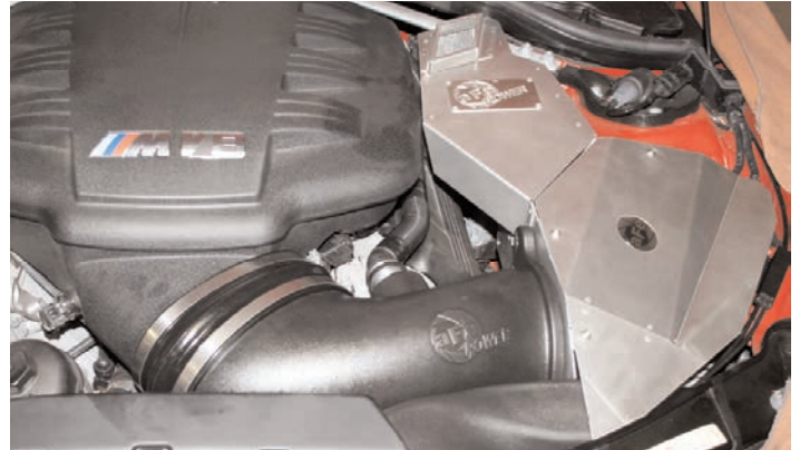
30- Place enclosed CARB EO sticker on a clean/smooth surface on or near the intake system. EO identification label is required in passing the Smog Check inspection. Your Installation is now complete. Please check all components and retighten if necessary. Thank you for choosing aFe Power!
