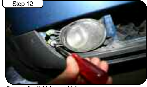
Step 12 Remove fog light from vehicle
