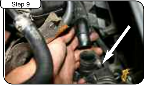
Step 9 Loosen clamp holding fourth breather down from top of tube with slotted screwdriver.
