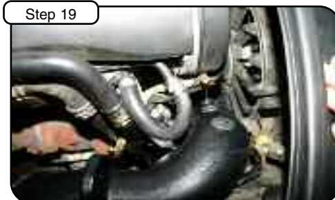
Slide tube coupling onto turbo. Tighten clamp at turbo end with 5/16" Nut driver. Install lowest breather onto large reduction barb fitting. Use provided #16 mini clamp.
