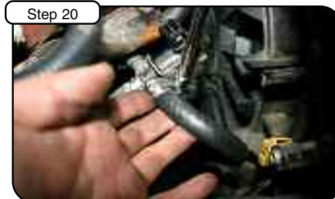
Use provided 8.5"L x 3/8" hose with 3/8" elbow and clamp. Install onto second from bottom fitting. Tighten clamp onto factory switch valve. Verify plug is reconnected.
