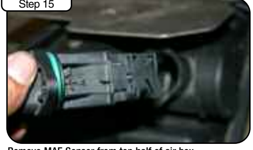
Step 15 Remove MAF Sensor from top half of air box.
