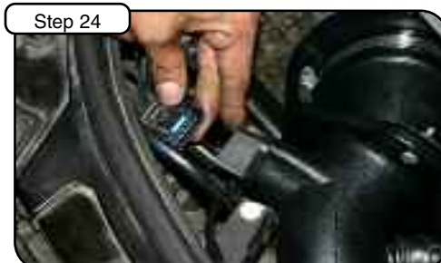
Re connect MAF Sensor plug
