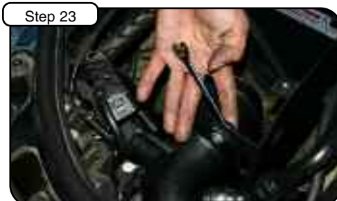
Align tube to housing and use provided M6x1x25 screw, M6 flat washer, M6 wavy washer, and M6 nut.
