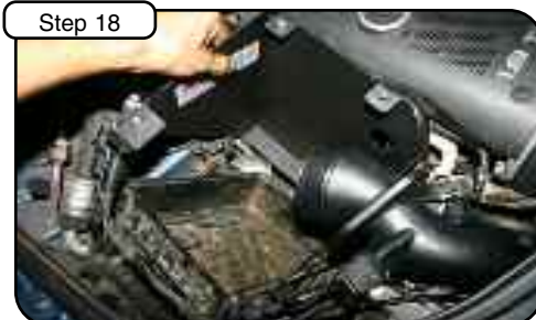
Place aFe housing and tube into vehicle. Align housing clip on base and align sides of housing to airbox.
