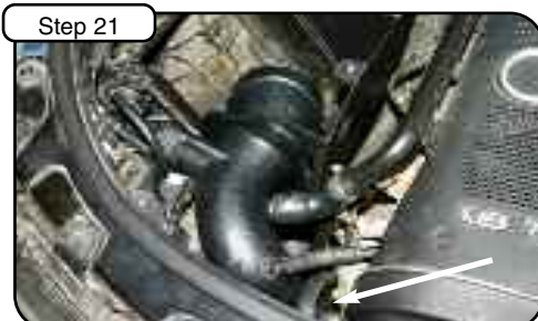
Install provided 22 "L x 3/8"D hose with 3/8" elbow onto third from bottom fitting. Route hose towards firewall area and clamp hose onto fitting.
