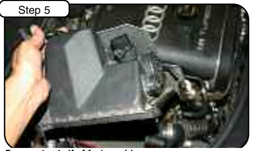
Step 5 Remove top half of factory airbox
