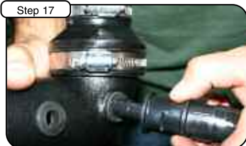
Install provided reducer coupler onto tube using provided clamps. Install two reduction fittings. Install larger reduction fittings onto grommet near turbo coupling. (Note: Use a lubricant to aid with installation) Install shorter reduction fittings on grommet nearest the MAF Sensor.
