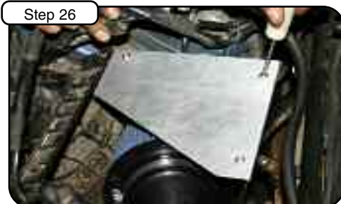
Install aFe cover using (3) M6x1x10 button head screws.
