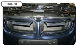
Your completed D.A.S. installation will look like this. Check and make sure they are secure. Re-install grills by lining up tabs and pushing them in until they snap into place.
