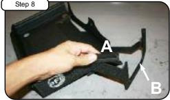
A) Attach 7/16" trim seal to top of housing.
