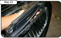
The grills are held in place with push clips. To remove, reach in behind each grill and push forward while using other hand to support grill fron the front.
