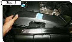
Pull back ram air duct and remove.
