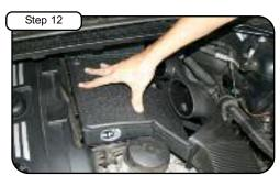
Push down housing allowing grommets to seat. Align threaded insert with hole on housing.
