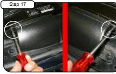
Remove screws on ram air duct using T25 torx bit. (Save for later installation)
