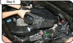
Remove complete air box from vehicle.
