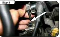
Remove clamps holding third breather filter from top of factory tube. Plug can be disconnected for ease of removal.
