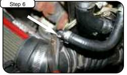
Remove clamp holding top breather filter on factory tube.
