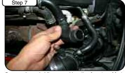
Remove clamps holding second breather from top of factory tube. Save elbow for later use.
