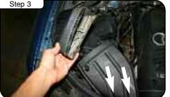
a. Remove two screws holding factory fresh air duct in place. b. Pull fresh air duct out of vehicle and save for later use
