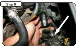
Loosen clamp holding fourth breather down from top of tube with slotted screwdriver.
