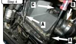
a. Remove two screws holding top half of airbox in place. b. Loosen clamp holding factory tube in place. c. Unplug MAF Sensor
