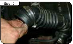
Loosen clamp at turbo and Last breather tube. Pull factory tube out of vehicle.
