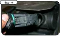
Remove MAF Sensor from top half of air box.
