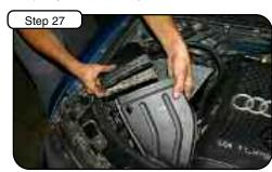
Install factory fresh air duct and tighten down two screws securing it to the core support.
