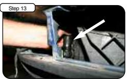
Disconnect Air pump hose at pump.
