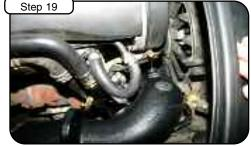
Slide tube coupling onto turbo. Tighten clamp at turbo end with 5/16" Nut driver. Install lowest breather onto large reduction barb fitting. Use provided #16 mini clamp.
