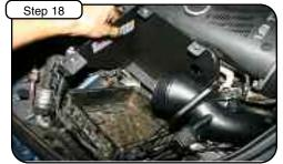
Place aFe housing and tube into vehicle. Align housing clip on base and align sides of housing to airbox.
