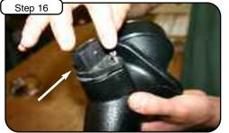
Using provided Gasket and (2) M4x.7x16 screws install MAF Sensor onto aFe intake tube.
