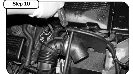
Place the new #044 clamp on the intake duct and tighten assembly to the housing inlet.
