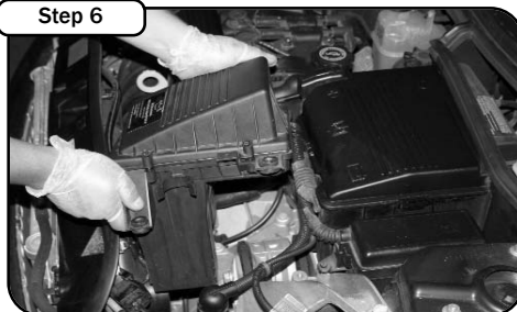
Remove the factory air box by grabbing the air box by the sides and lift up and out.
