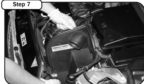
Position the new housing into the engine bay. Place the trim seal along the edge of the housing.
