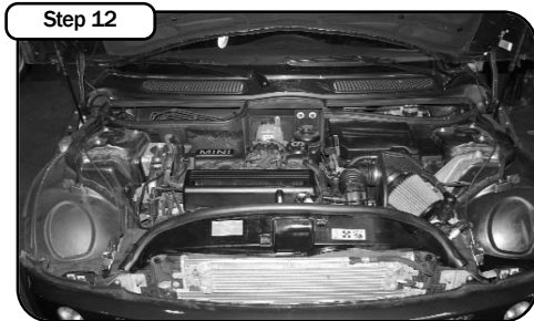
Place enclosed CARB EO sticker on a clean/smooth surface on or near the intake system. EO identification label is required in passing the Smog Check inspection. Your installation is now complete. Make sure you tighten all clamps and check all electrical connections. Re check periodically.
