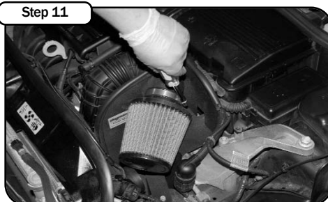
Install the new air filter into the housing secure the filter with the provided clamp. The air filter is pre oiled from the factory. Do not use any grease or oil.
