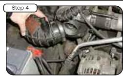
Remove factory rubber elbow at turbo.
