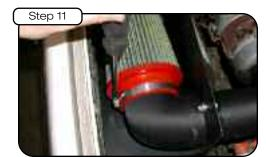
Install provided aFe filter onto the plastic tube and tighten.
