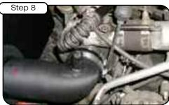
Tighten the remaining clamp securing the tube to the turbo coupler.
