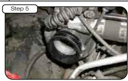
Place provided coupler onto turbo and secure the turbo end by tightening provided clamp.
