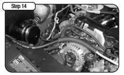
Install provided couplers. Be sure to install the small end of the tapered coupler to the turbo inlet Induit in portical cooper to a size of the state in the state of the coper to cooper to the too inter-housing. The remaining coupler too is installed with the smaller inner diameter attached to the heat shield, and the larger inner diameter will receive the Stage 2 tube. Install Stage 2 tube into couplers. Reposition duct clamps if additional clearance is necessary.
