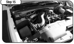
Complete Stage 2 kit installed. Make sure all clamps are tight and all components are secure. Check and retighten connections and filter after a few hours of operation.
