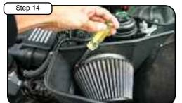
Install your high FLOW air fliter. Tighten using 5/16" nut driver.
