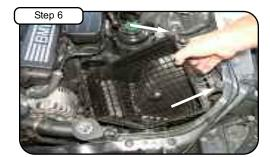
With T25 torx bit, loosen the 2 bolts holding bottom half of OE airbox. Take out OE airbox. Save bolts for later use for install.
