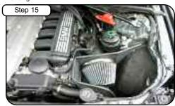
Place enclosed CARB EO sticker on a clean/smooth surface on or near the intake system. EO identification label is required in passing the Smog Check inspection. Your installation is now complete. Check all clamps and hoses periodically. Thank you for choosing a Fe!
