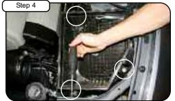
Loosen the 3 bolts holding in bottom half of air box. Take air box out of vehicle.
