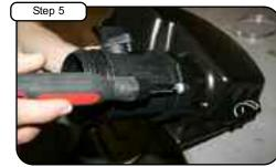
Remove MAF sensor using T30 torx bit.
