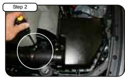
Disconnect MAF sensor harness. Loosen clamps with 1/4" nut driver.
