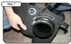
Install coupler reducer to filter adapter with clamps provided.
