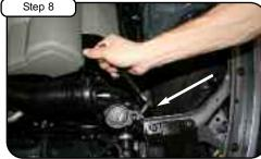
With 10mm socket loosen the bolt holding in windshield washer resevoir. Save bolt for later install.
