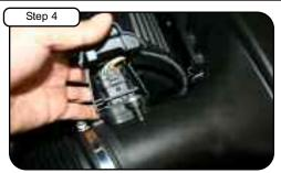
Remove te MAF sensor cover. Disconnect the MAF harness from sensor
