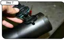
With provided T20 torx bit loosen the 2 bolts that hold in the MAF sensor. Carefully remove MAF sensor out.
