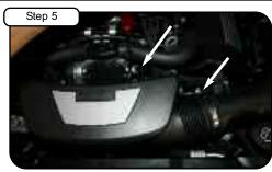
With 1/4" nut driver loosen the OE intake tube from throttle body and airbox. Remove intake tube out of vehicle.
