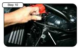
With OE T25 bolt, use to tighten new housing in to place. Tighten at botton of housing using nut and washer provided with 10mm socket w/ extension.
