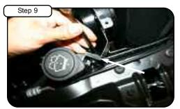
Using a 10mm wrench loosen bolt holding washer fluid resevoir. Place 5 1/2" adapter in to new housing and tighten using button head screws provided with 5/32 allen key. Install housing in to vehicle and re-tighten bolt
