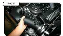
Place couplers with clamps provided on to tube and install new tube in to vehicle.
