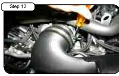
Tighten clamps using 5/16" nut driver.
