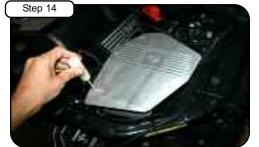
Place high FLOW filter into housing and tighten using 5/16" nut driver. Install housing cover using the 3 button head screws and tighten using 5/32" allen key.
