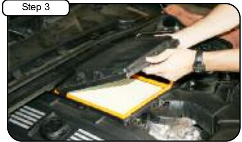
Unclip upper half of air box to remove lid and filter.
