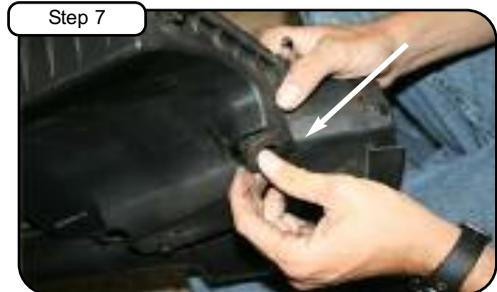
Remove the 3 rubber grommets from the air box. (To be used in step 9.)
