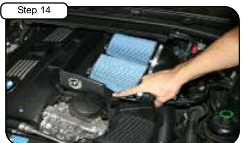
Install air filters and tighten with 5/16" nut driver and connect vacuum line.
