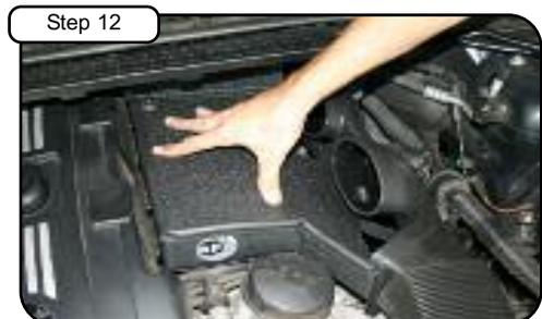
Push down housing allowing grommets to seat. Align threaded insert with hole on housing.
