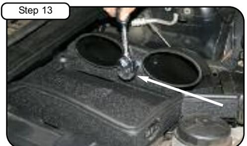
Install screw, washer and wavy washer provided, and tighten with 10mm socket or wrench. Tighten clamps to tube with 1/4" nut driver.
