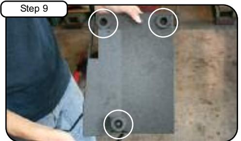
Install rubber grommets from step 7 on new housing.
