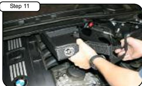
Install housing into factory position.
