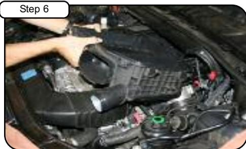
Remove complete air box from vehicle.
