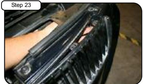
The grills are held in place with push clips. To remove, reach in behind each grill and push forward while using other hand to support grill from the front.
