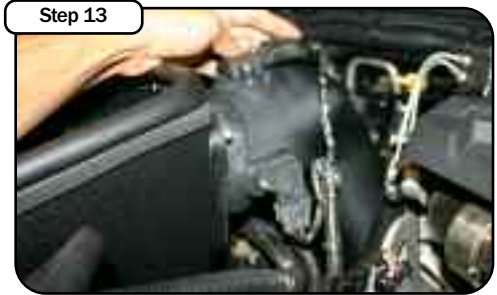
Step 13 Now tighten clamp at OE coupler and tube using 5/16" nut driver. Connect MAF sensor and temp sensor.
