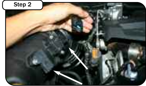
Step 2 Disconnect MAF sensor and temp sensor harness.
