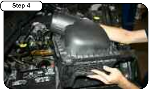
Step 4 Loosen the 10mm nut at front of air box and remove. Carefully grab and pull out OE intake system from vehicle.
