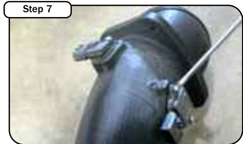
Step 7 Insert MAF sensor and temp sensor into new tube with gaskets and #8-32 screws provided. Tighten using flathead screwdriver.
