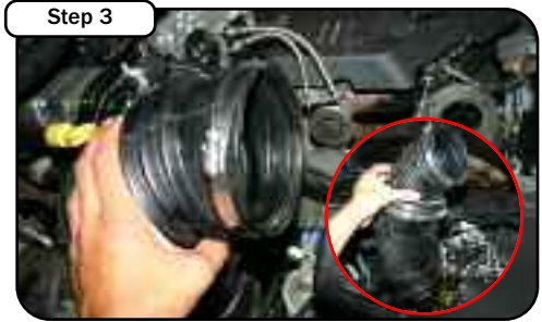
Step 3 With 5/16" nut driver, loosen the clamp at air box and at bottom of intake tube. (Make sure NOT at turbo!) Remove upper half of OE intake tube and leave bottom OE coupler.
