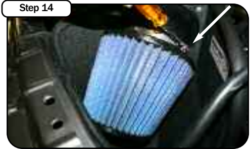
Step 14 Install air filter and tighten using 5/16" nut driver. NOTE: Place enclosed CARB EO sticker on or near the Intake on a smooth/clean system. EO Identification label is required to pass the smog test inspection.
