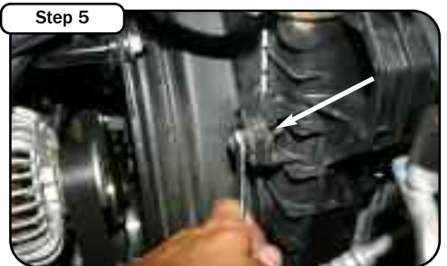
Step 5 Loosen and remove the 13mm radiator bolt. Set aside for later use.
