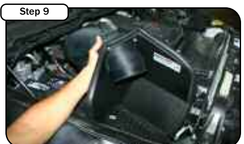
Step 9 Install new housing with intake tube into vehicle. Position tube and housing to factory position.
