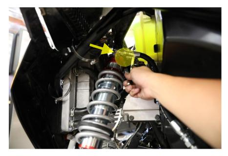
15. With the jack still under the lower arm, place the lower mount in its location and install and tighten the 15mm bolt and nut.
