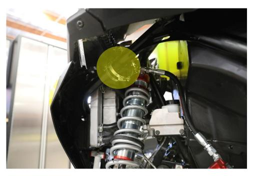
17. Put the reservoir in the location seen below and tighten the hose clamps with the rubber mounts between the reservoir and cage tubing.
