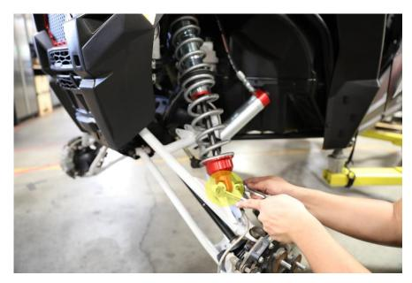
16. Prepare the supplied rubber mounts and hose clamps by loosening the hose clamps and installing them around the tubing as shown.
