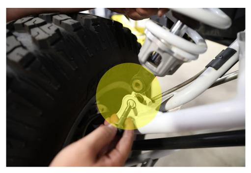
10. Remove the 15mm bolt and nut from the upper mount.
