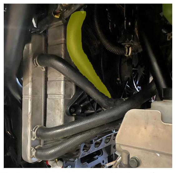
13c. While making sure the radiator hose does not move, re-install the bracket removed from step 13a.
