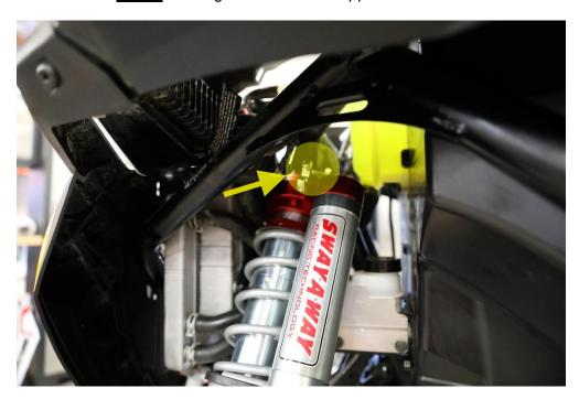
13a. Loosen the 10mm bolt holding on the highlighted bracket.
