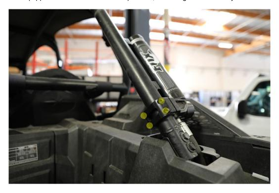
10. Lower the reservoir through the opening and let the reservoir rest where comfortable.
