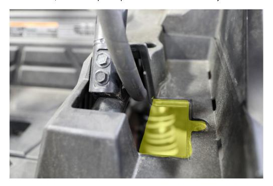
9. Locate the remote reservoir mount and use the 5mm allen wrench to remove the 4 screws holding on the reservoir.
