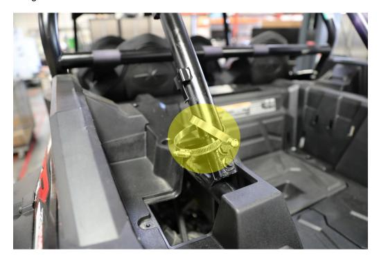
20. Put the reservoir in the location seen below and tighten the hose clamps with the rubber mounts between the reservoir and cage tubing.
