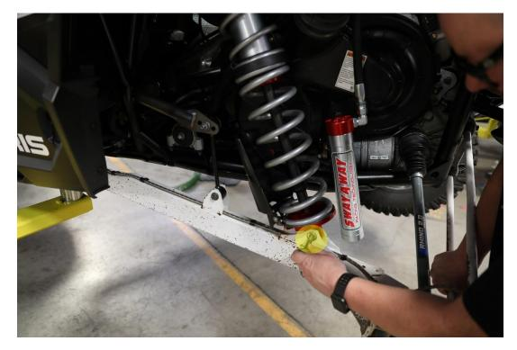
18. With the coilover fully mounted, pass the reservoir through the pass through location.
