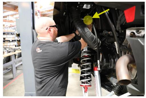
17. With the jack still under the lower arm, place the lower mount in its location and install and tighten the 18mm bolt and nut.
