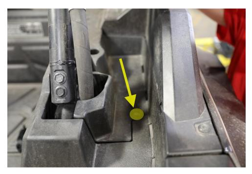
8. Loosen the T20 torx screw, remove the plastic panel and move out of the way.
