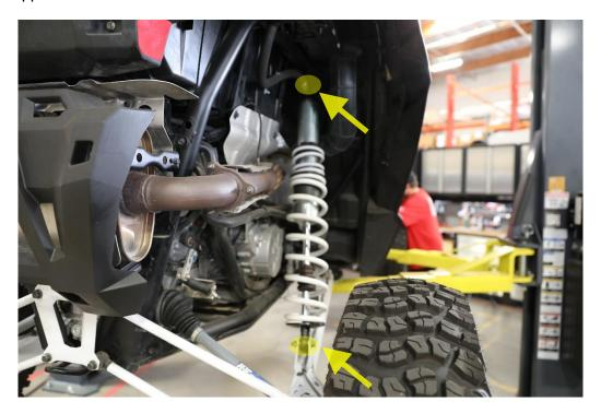
12. Beginning with the lower mount, use the 18mm open end wrench and 18mm socket to remove the lower bolt
