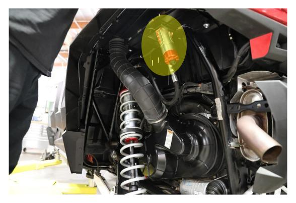
19. Prepare the supplied rubber mounts and hose clamps by loosening the hose clamps and installing them around the tubing as shown
