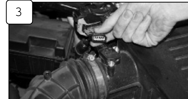
Disconnect MAF sensor harness. With Phillips or 10mm socket or wrench loosen both clamps on intake tube.
