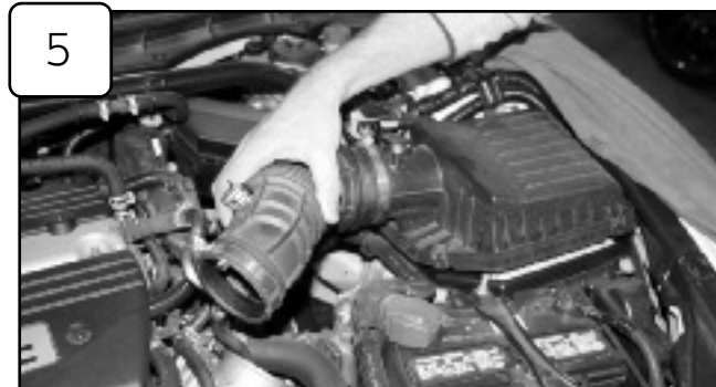
Un-clip upper half of air box and remove stock intake.
