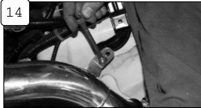
Using isolation mount provided, secure to vehicle and position tab on tube to isolation mount. Tighten using the washer and nut provided with 10mm socket or wrench.
