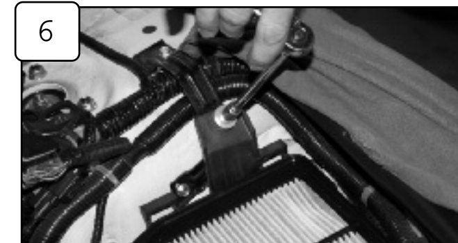
Loosen bolt securing in bottom half of air box using 10mm socket or wrench and remove along with air filter.
