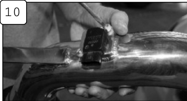
Install MAF sensor to intake tube using provided M4 screws.
