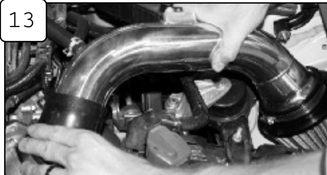
install intake tube assembly into vehicle and position.
