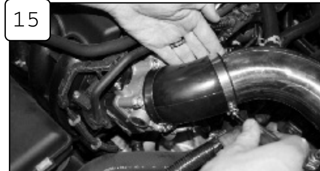
Position and tighten clamps on tube using 5/16" nut driver.
