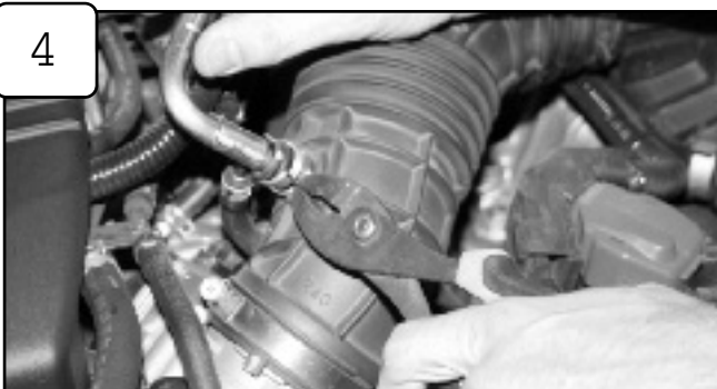
With pliers remove crank case line from intake tube.
