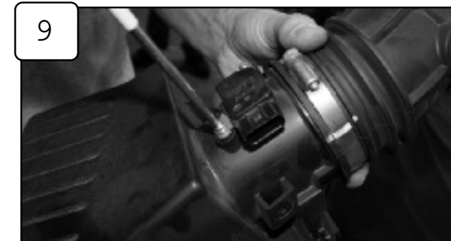
Remove MAF sensor from stock air box using phillips screwdriver.
